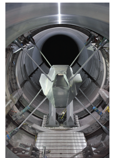
JF12试验模型-吸气式高超声速飞行器内外流一体化性能试验 A test model of JF12 - A hypersonic air-breathing vehicle for the integration performance study on inner/outer flow interaction
