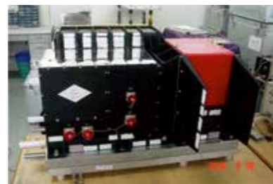
风云三号卫星红外分光计 InfraRed Atmospheric Sounding Interferometer (IRAS) on-board FY-3 satellite
