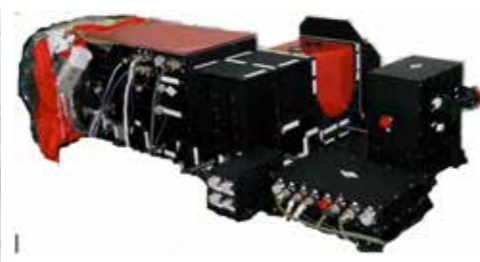
风云三号卫星中分辨率光谱成像仪 MEdium Resolution Spectral Imager (MERSI) on-board FY-3 satellite
